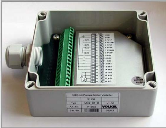
The electric connection is established using the terminal block in the housing. A 9-pin socket serves for the connection to a PC, alternatively to the MT mini terminal. The current equipment status (supply voltage, communication, inputs/outputs) can be checked via the die integrated LED.
